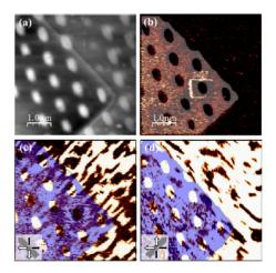
Nanoislands milled out of a BFO lamellar structure via a process of repeated ion milling. a) Topography, b) vertical PFM phase, c), d), lateral PFM phases, orthogonal to each other.<sup>[2]</sup>
