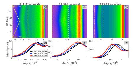
Using this technique, we demonstrated that effective piezoelectric coefficient  $d_{33}$  of the MFP phase ranges between 60 and 100 pC / N [2]. This large value of piezoelectric coefficients motivates for further studies with the ultimate goal of shifting the effect from the near-surface layer to the bulk.
